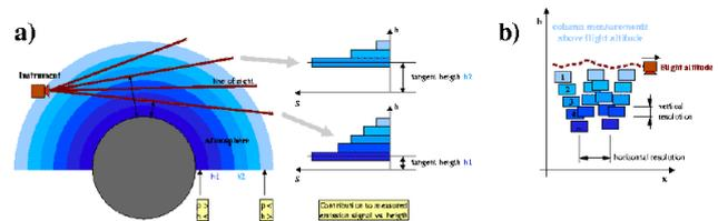
Fig. 3: The limb sounding observation geometry. a) vertical resolution. b) horizontal resolution.
