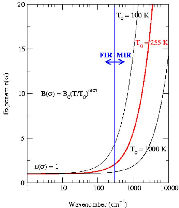
Fig. 2: Temperature dependence of the Planck function.
