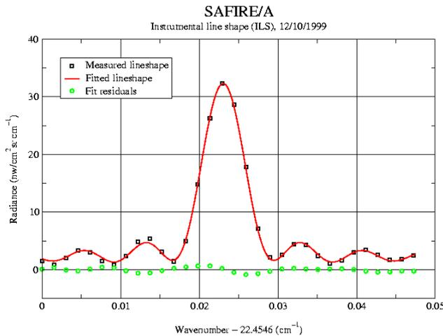
Fig. 10: Instrumental Line Shape (ILS) of the SAFIRE/A spectrometer.
