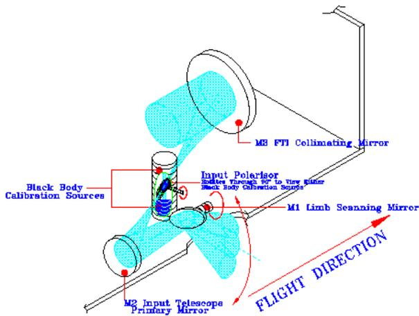
Fig. 6: Schematic of the SAFIRE/A input optics.
