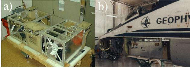
Fig. 9: Photographs of the SAFIRE/A instrument. a) instrument ready for laboratory operations. b) instrument installed on the M55 Geophysica.
