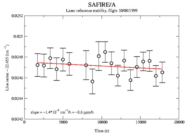
Fig. 11: Frequency stability of the SAFIRE/A laser reference system.
