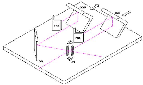
Fig. 7: The SAFIRE/A FIR interferometer
