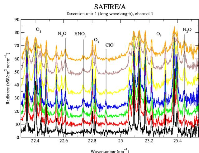
Fig. 14 - Limb-scanning sequence of atmospheric emission spectra acquired in the 22-23.5  $\text{cm}^{-1}$  window. Spectral features due to interesting molecular species are evidenced by vertical lines.
