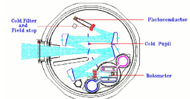
Fig. 8: The Cold Optics and Detector Module (CODM).
