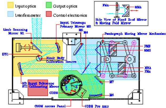
Fig. 5: The SAFIRE/A spectrometer, optical layout.
