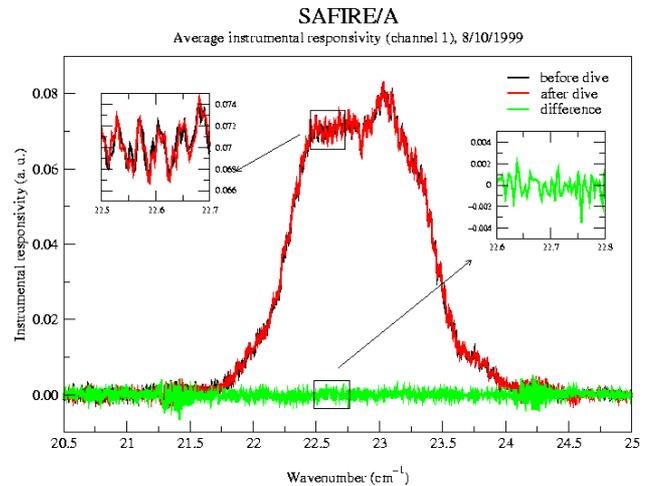
Fig. 12: Radiometric calibration stability of the SAFIRE/A spectrometer.
