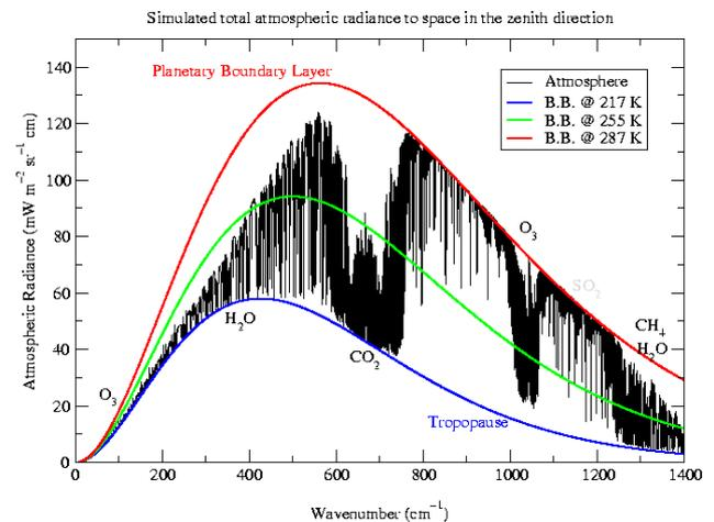
Fig. 1: Simulated emission spectrum of the earth's atmosphere in the zenith direction.
