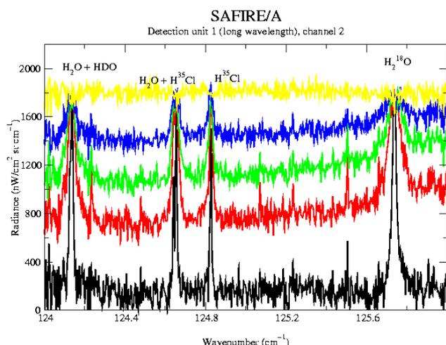
Fig. 15 - Limb-scanning sequence of atmospheric emission spectra acquired in the 124-126 cm<sup>-1</sup> window. Spectral features due to interesting molecular species are evidenced by vertical lines. Atmospheric opacity due to water vapour absorption limits analysis to upper atmospheric layers, so only limb scanning angles corresponding to upper layers are presented.
